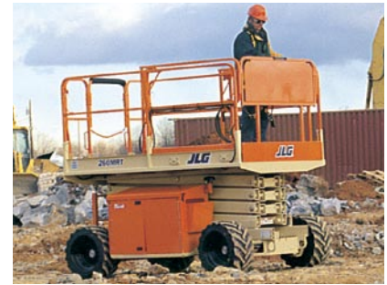
Standard Cross Corner Four-Wheel Drive for Terrainability
